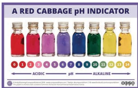
Figure 1. The pH scale for a red cabbage pH indicator.
